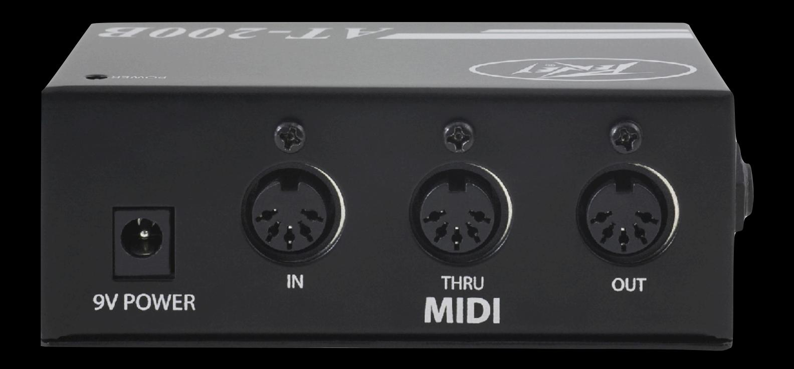
MIDI standardized the control signal and inter-machine communication between synthesizer devices using inexpensive, readily available cables.
