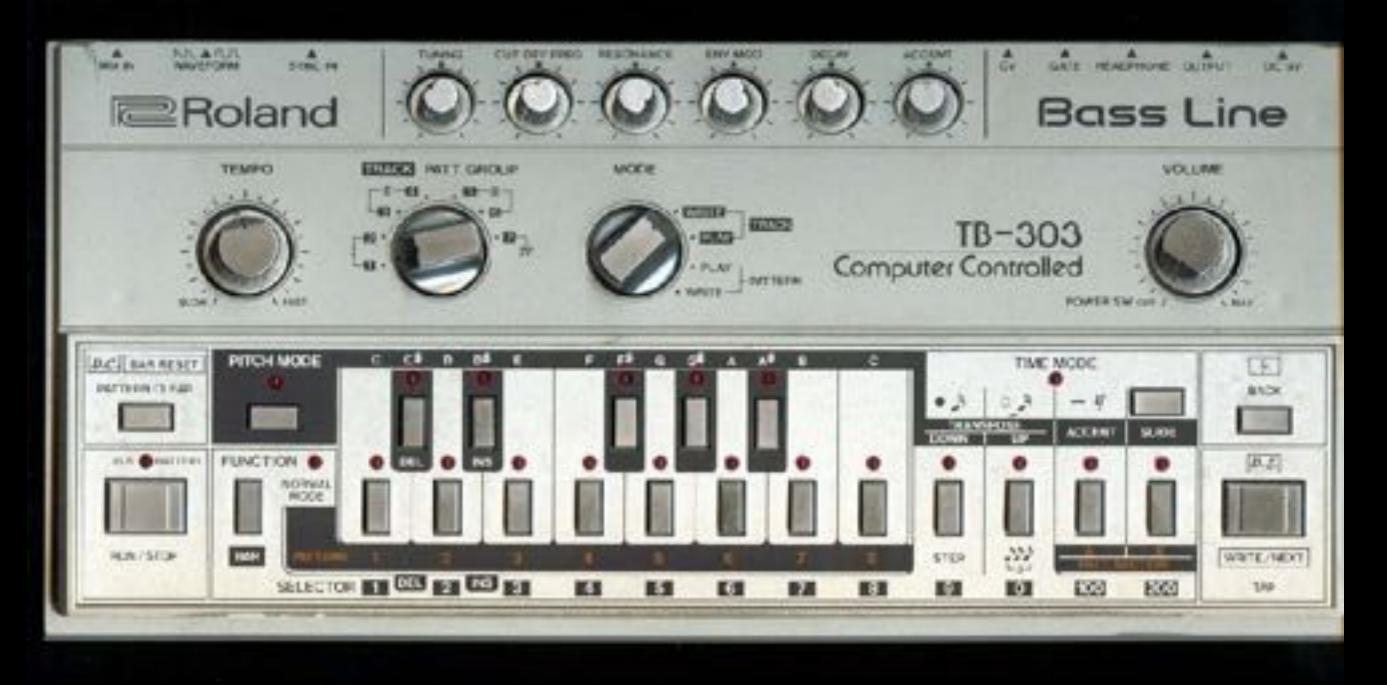
The Roland TB-303 Bass Line Synthesizer, released in 1982, was a commercial failure and was only in production for 18 months. In the late 1980's these boxes, now inexpensive, were repurposed to create Acid. The upper knobs could be controlled to change the timbre on a repeating patter, adjusting a VCF - resonance, filter cutoff and envelope. Other knobs controlled tuning, decay, and accent.
